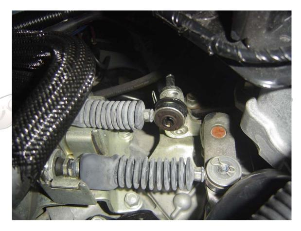
3. Remove both 12mm bolts holding shift bracket to the transmission and remove bracket. Be sure not to drop the white plastic slider that goes to the main shift rod.
