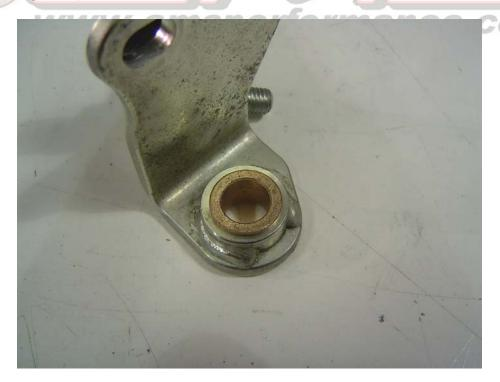
7. Lube the arm piece of the bracket and reinstall into new bushing, if movement is slightly tough at first move the arm around inside the bracket, movement will smooth out.
